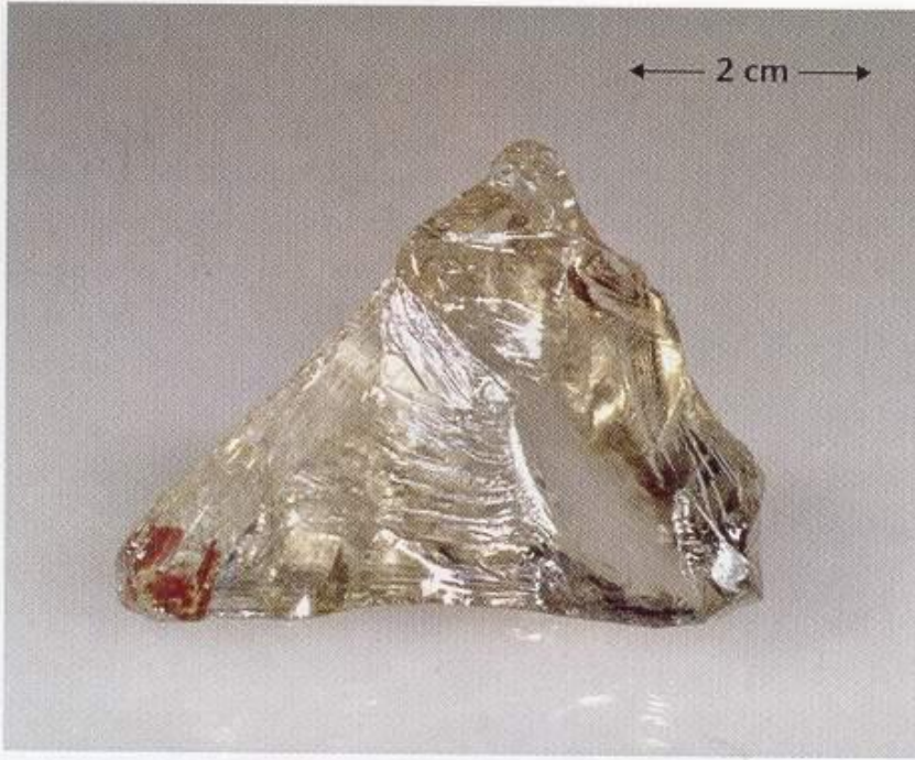
Figure 2.14 Conchoidal fracture. The smooth curved surfaces result when minerals break in a glasslike manner. (Photo by E. J. Tarbuck)
