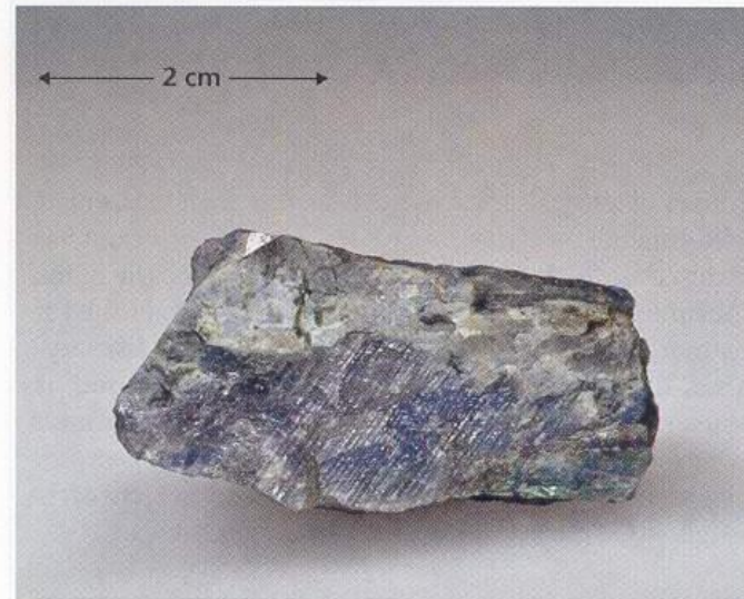
Figure 2.24 These parallel lines, called striations, are a distinguishing characteristic of the plagioclase feldspars. (Photo by E. J. Tarbuck)
