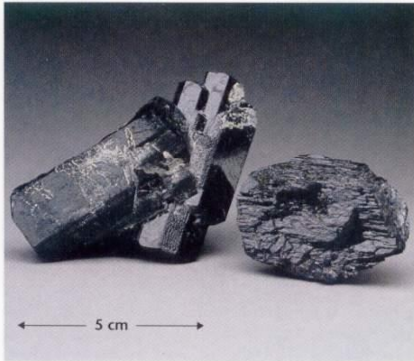
Figure 2.20 Hornblende amphibole. Hornblende is a common dark silicate material having two cleavage directions that intersect at roughly 60^\circ and 120^\circ .
