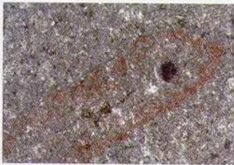
Figure 3.18 These dark-colored mafic rocks are composed primarily of pyroxene and calcium-rich plagioclase. A. Basalt is aphanitic and a very common extrusive rock. B. Gabbro, the phaneritic equivalent of basalt, is less abundant. (Photos by E.J. Tarbuck)
