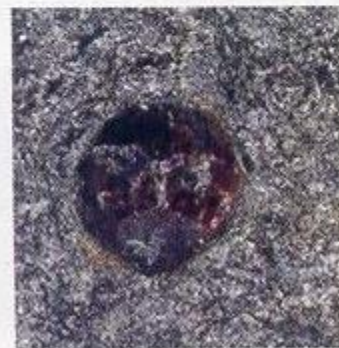
Figure 7.10 Garnet-mica schist. The dark-red garnet crystals and the light-colored mica matrix formed during the metamorphism of shale. (Photo by E. J. Tarbuck)
