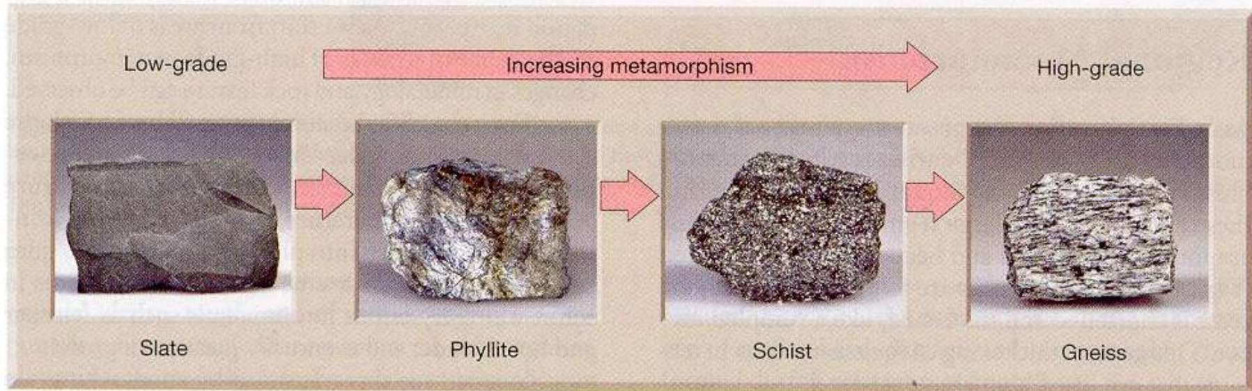
Figure 7.17 Idealized illustration of progressive regional metamorphism. From left to right, we progress from low-grade metamorphism (slate) to high-grade metamorphism (gneiss). (Photos by E. J. Tarbuck)
