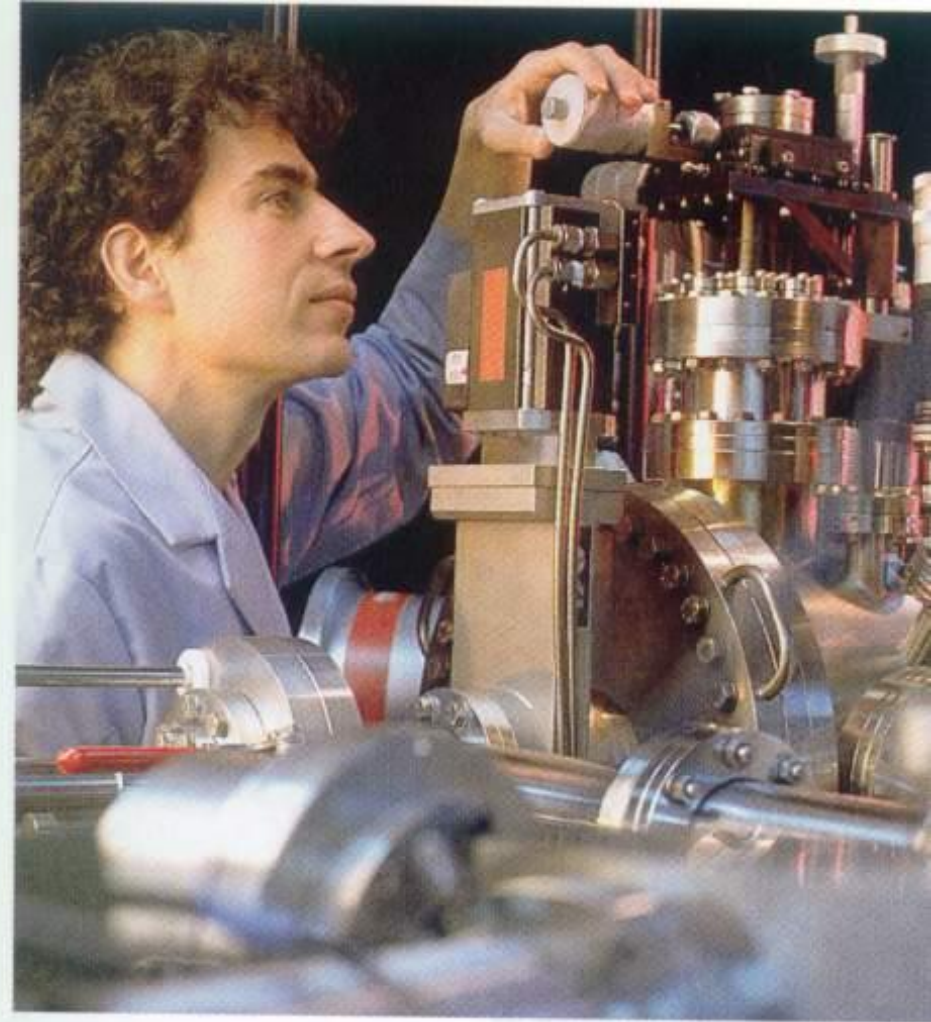
Figure 1.8 This scientist is using a mass spectrometer to analyze rare gases for geophysics research. (Photo by Jean Miele/The Stock Market)
